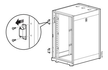
6. Reinstall the hinges on the opposite side of the enclosure.
